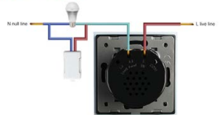
If there is neutral line inside the mount box, it can be directly connected as...
